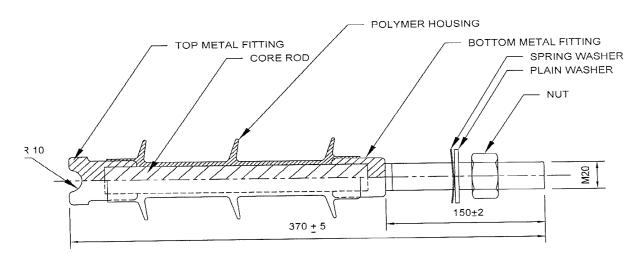
Diameter of FRP rod - 24 mm (minimum) Arcing distance - 165 mm( minimum)
